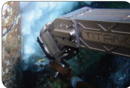
SubC Control's 1Cam takes 12.3 megapixel stills and 1080p video and records them to its internal memory. It also offers live high definition images. Shown here, a HD image of an underwater cleaning operation and a sea slug in the Gulf of Mexico.
